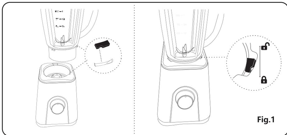
4. Place the lid on the jug and press to secure. Place the measuring cap into the hole in the lid and turn clockwise to lock.
