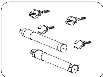
③ Make a hole at the installation position (200mm distance between holes). Put a fish-shaped screw plug into the hole and knock it into place, then fix the T8 tube to the wall with a self-tapping screw and fasten the tube into the clip.
