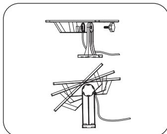
② Fix the solar panel on the bracket with a screw by hand. Adjust the angle: the face of the photovoltaic panel towards 5-10 degrees west to south and at a certain angle to the horizontal (30 degrees in the south, 45 degrees in the north), and twist it tightly.
