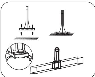
① Make a hole at the installation position (according to the distance between the holes of the bracket). Insert the fish-shaped screw plugs into the holes and knock them into place, and install the bracket with self-tapping screws; or tie the bracket at the installation position with a tie.
