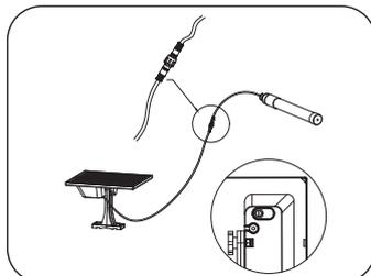
④ Connection: plug in the male and female plugs and tighten the waterproof nuts. Check and secure after installation. Press the switch on the back of the power box and remove the PVC spacer at the end of the remote control to control the working mode of the luminaire.
