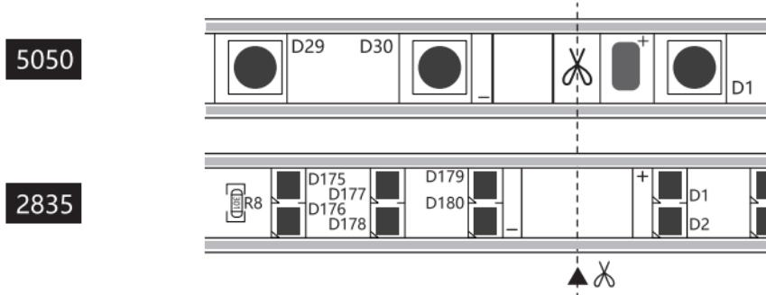
Cutting the strip to the length which you need from the cutting mark here (or from the space between every 1 meter); sometimes the strips are not with the cutting mark, but it must have obvious spacing which is wider than other points.
